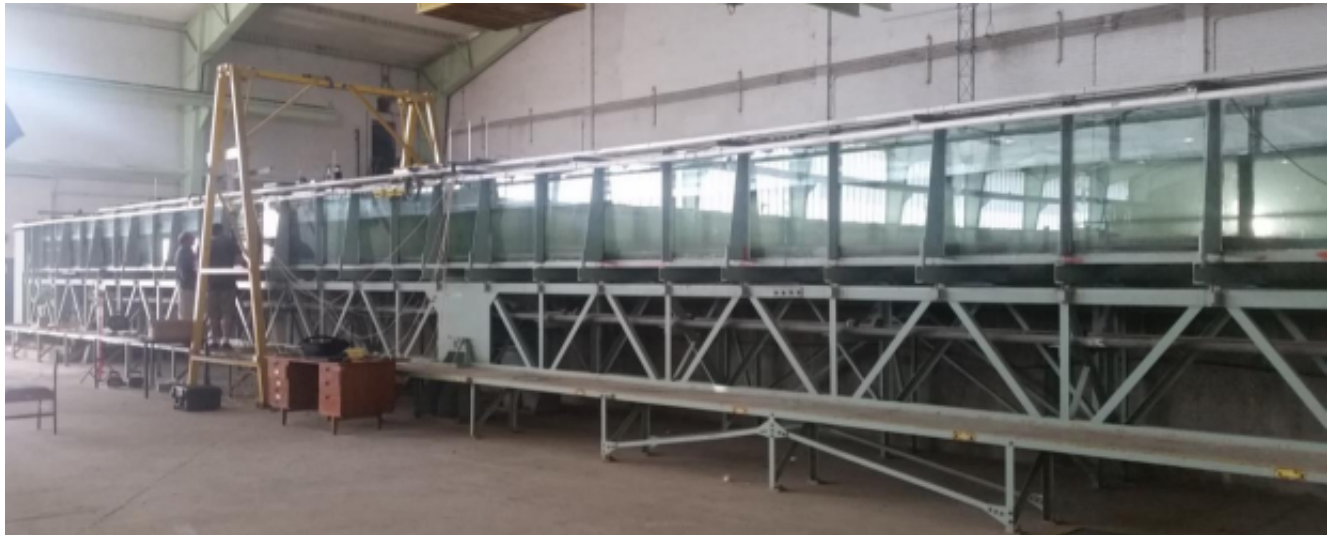
Figure 4.1: Glass flume at the CSIR Coastal and Hydraulics (Terblanche et al., 2018)
